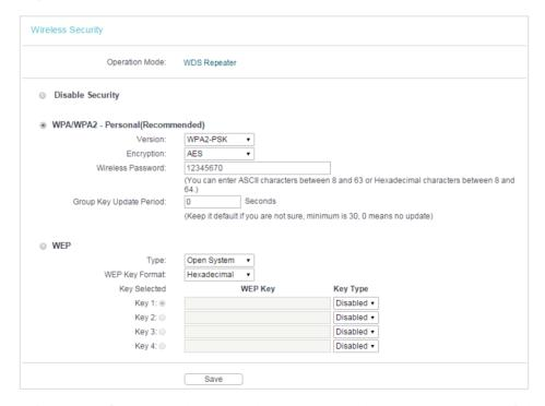
Disable Security - Check this box radio button to disable wireless security. If disabled, the wireless stations will be able to connect this device without encryption. It is strongly recommended that you choose one of the security types to enable security.
