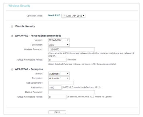
You can choose which SSID to configure wireless security settings for in the blank behind Operation Mode.
