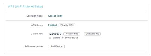
2. Enter the access point's current PIN on your client device to join the access point's Wi-Fi network.
