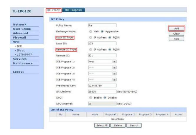
NOTE: No matter on Main mode or Aggressive mode, once the client PC is behind a NAT device, we have to select FQDN as ID Type and the NAT device must support VPN passthrough, otherwise the VPN tunnel can't be established.
