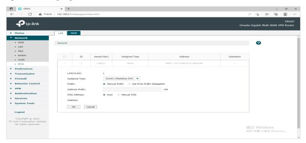
Figure 8-12 Configuring the SLAAC+Stateless DHCP
