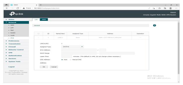
Figure 8-10 Configuring the SLAAC+Stateless DHCP
