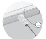
Note: For lightning and ESD protection, connect the EAP's grounding terminal to grounding facilities using a proper grounding wire, which should meet local installation requirements.
